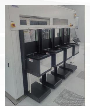
Mechatronics Wafer Sorter 4x PLM 200W on Boltnterface
